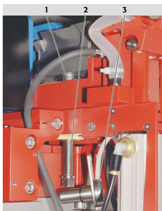
Fig. 47 Furnace shroud, partly pressed out
