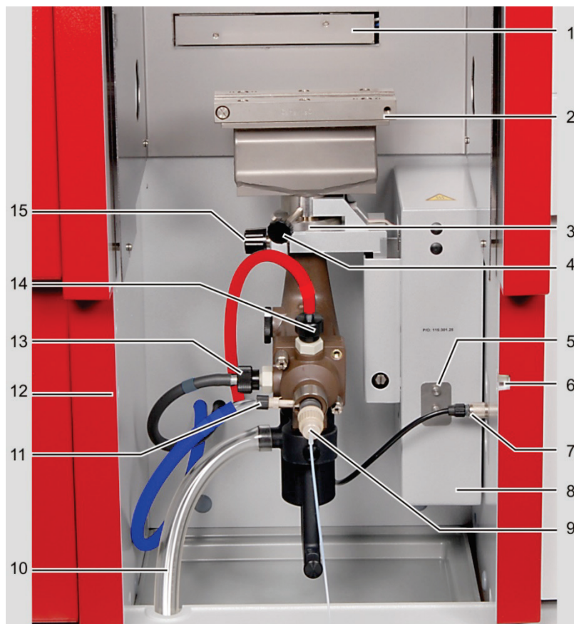
Fig. 38 Connections to the burner-nebulizer system in the sample chamber
