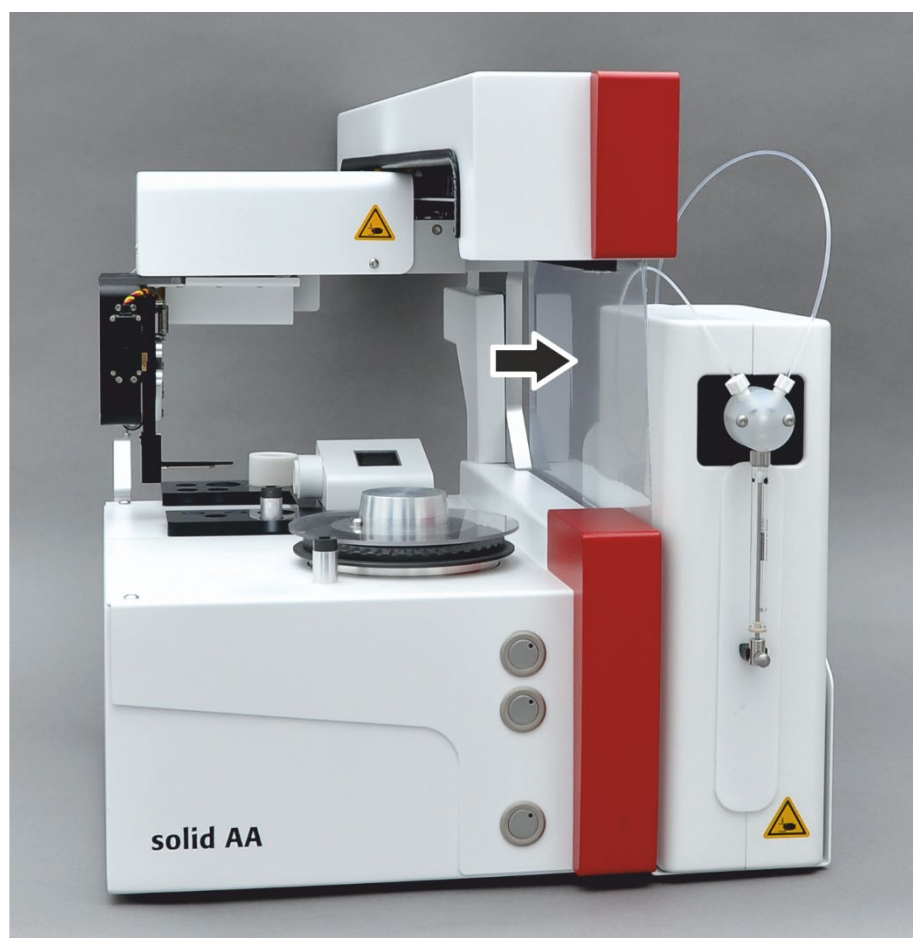
Figure 21 Protective film at the SSA 600 (arrow)
