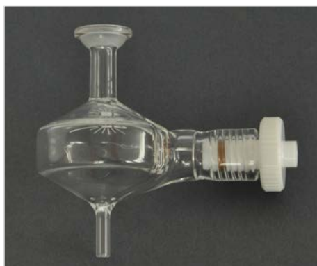
Fig. 2 Cyclonic spray chamber 20 mL
