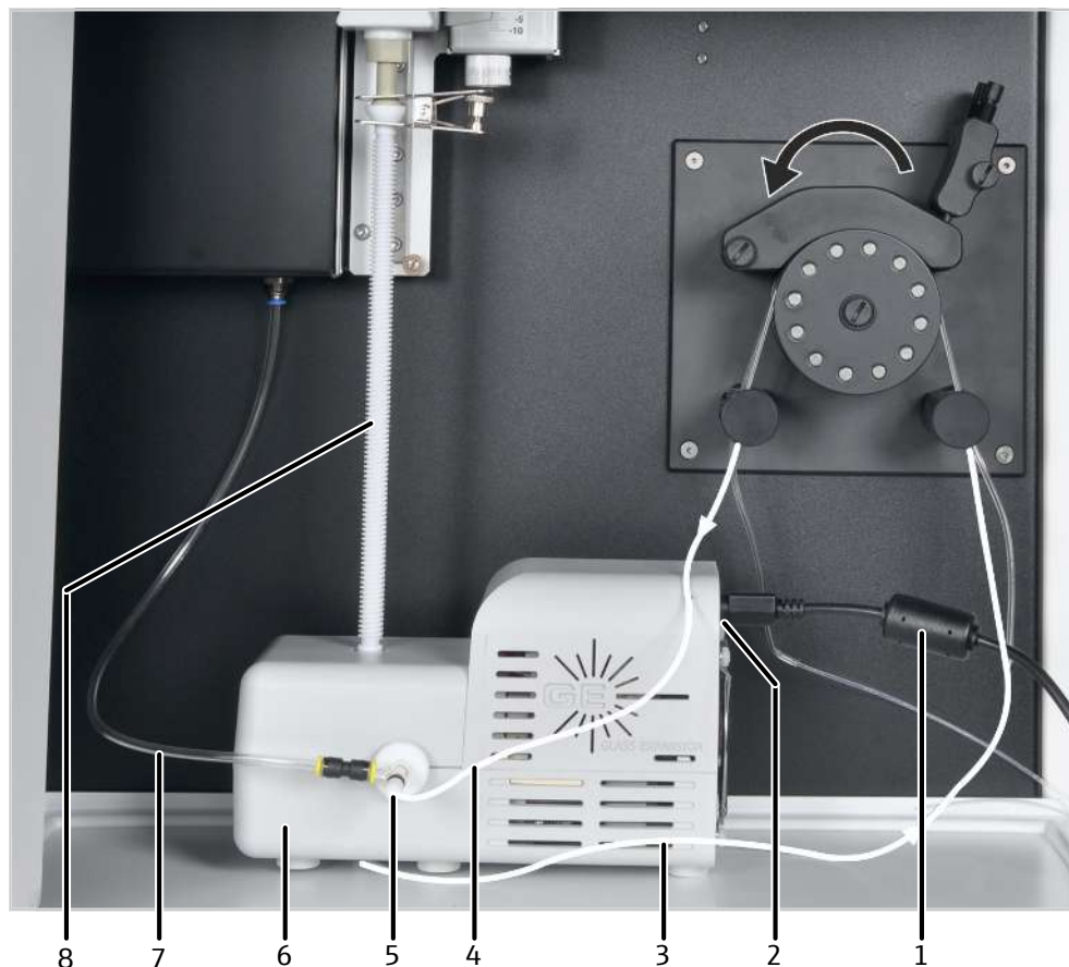
Fig. 25 Installing the temperature-controlled spray chamber
