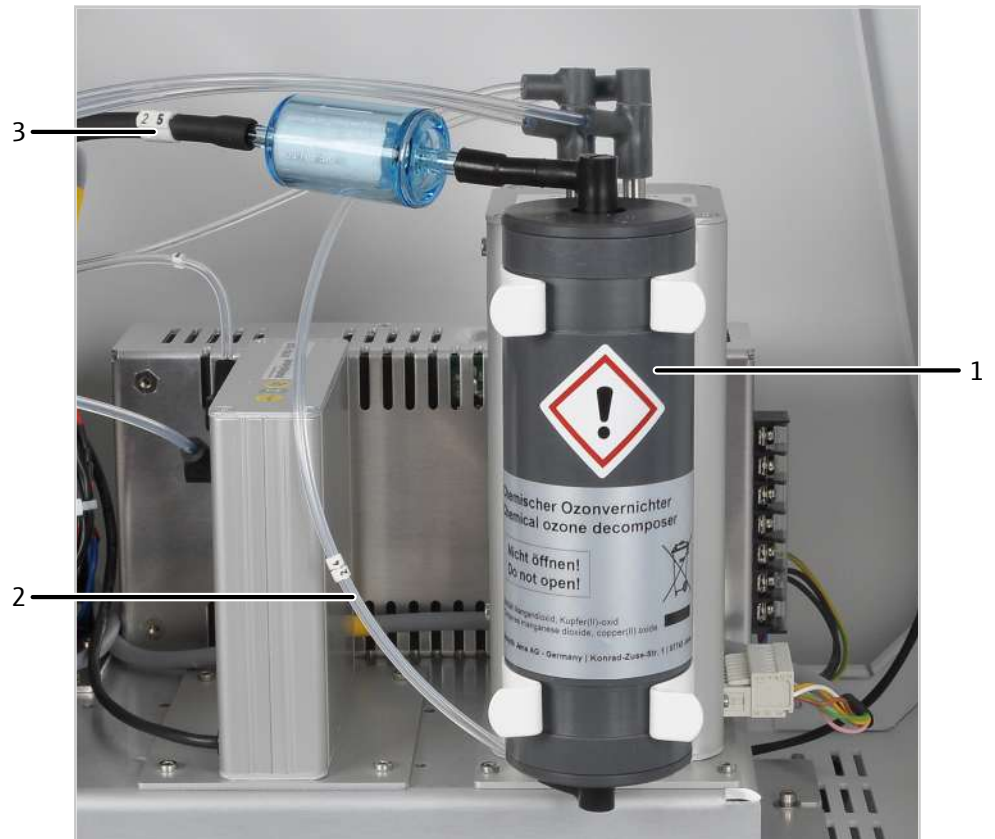
Fig. 70 Replacing the chemical ozone decomposer
