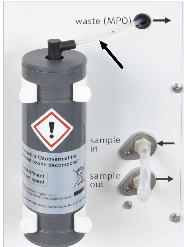
Fig. 73 Replacing the chemical ozone decomposer
