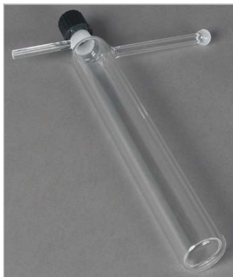
Fig. 58 TOC combustion tube (unfilled)
