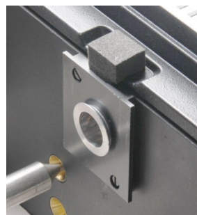
Fig. 103 Reflector inserted into the adapter for the cell holder
