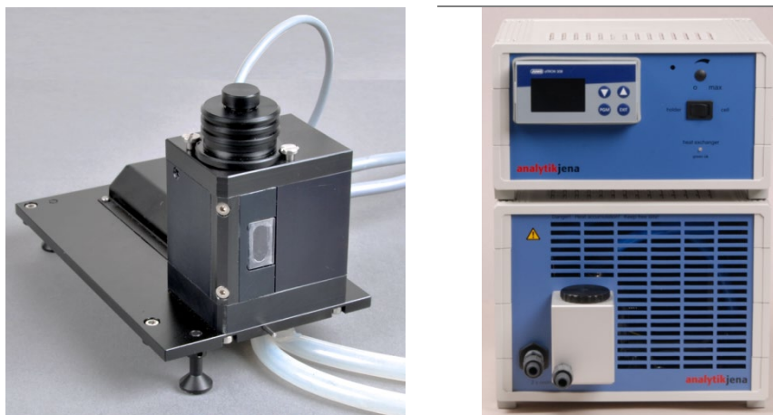
Fig. 54 Peltier-tempered cell holder with temperature control unit and heat exchanger
