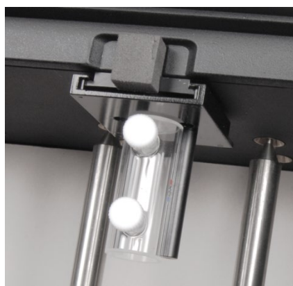
Fig. 25 Holder for cylindrical cells installed in the SPECORD PLUS
