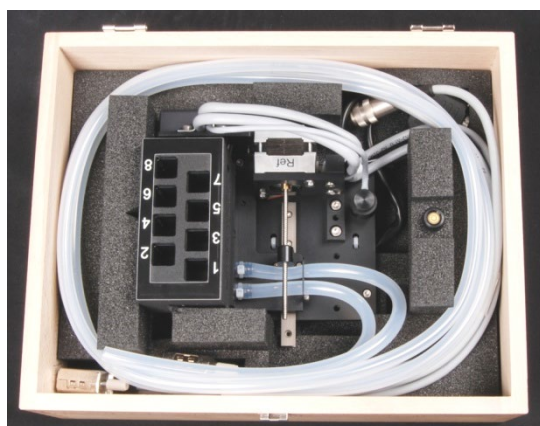
Fig. 61 Peltier-tempered 8-cell changer in the storage container
