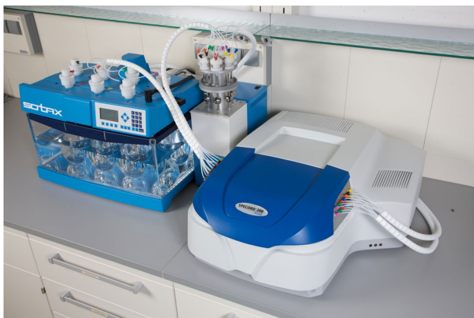
Fig. 86 The SPECORD PLUS with connected Dissolution system
