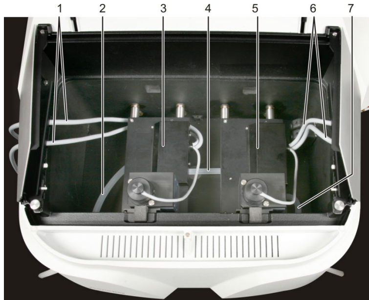
Fig. 57 Two cell holders (Peltier-tempered with heat exchanger) installed in the sample chamber
