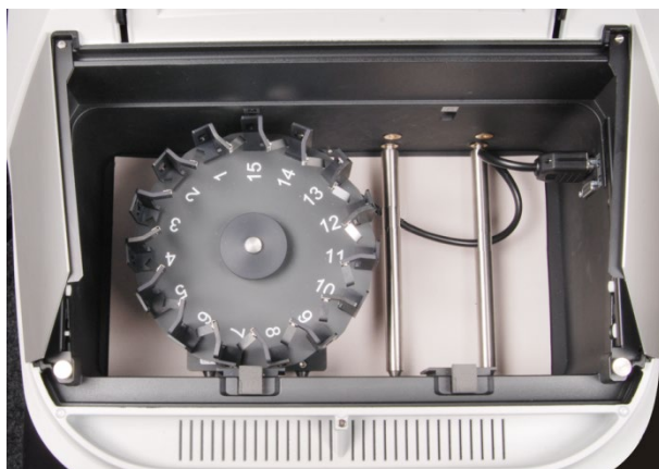
Fig. 39 Cell carousel fully mounted
