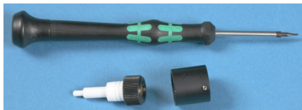
Fig. 48 Conversion kit for ultra-microcells
