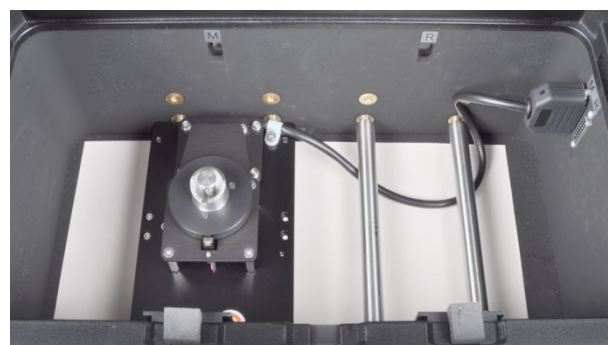
Fig. 38 Base plate of the cell carousel installed in the SPECORD PLUS
