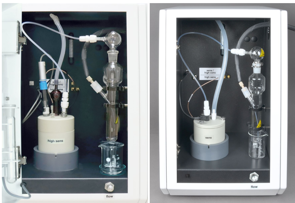
Measuring cell "high sensitive"
