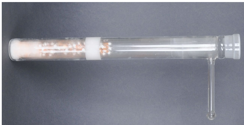
Fig. 13 Combustion tube filled with used quartz containers
