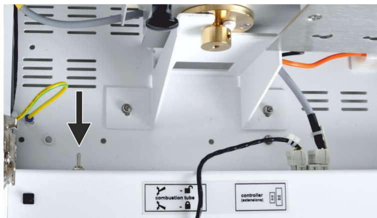
Fig. 17 Toggle switch to lock/release combustion tube
