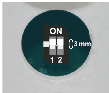
Gas sampling system as last module: DIP switches 1 + 2 in the upper position "ON" (factory default setting)
