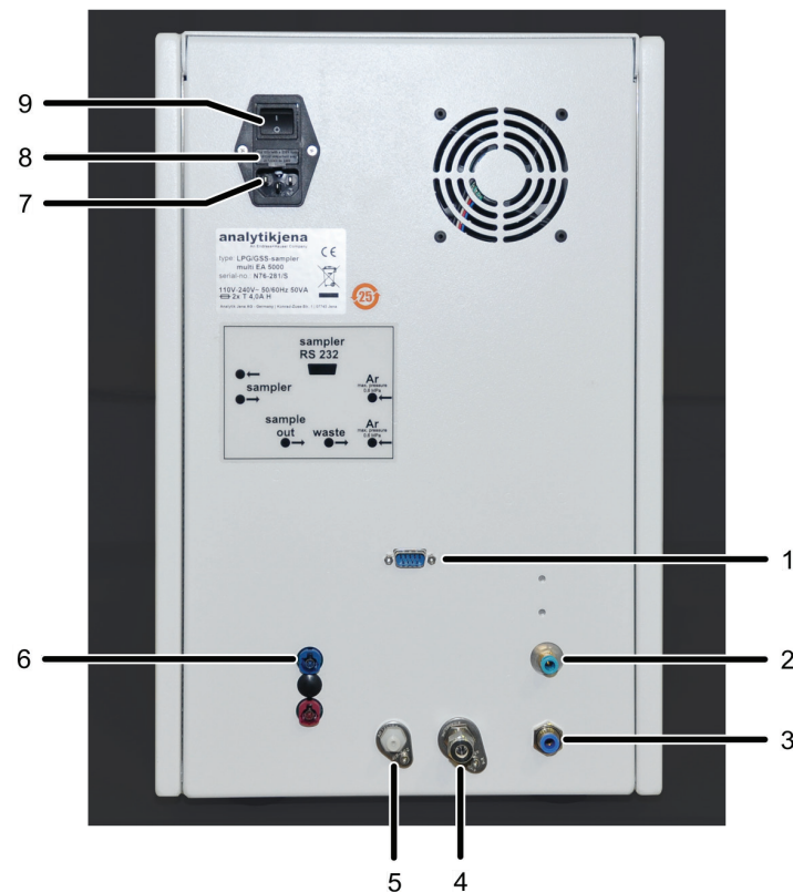
Figure 7 Device backplate of the GSS/LPG combi module with interfaces and device switch
