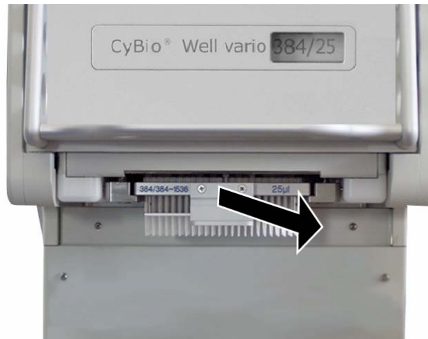
Fig. 91: Remove tip magazine or capillary magazine (head replacement from the front version)
