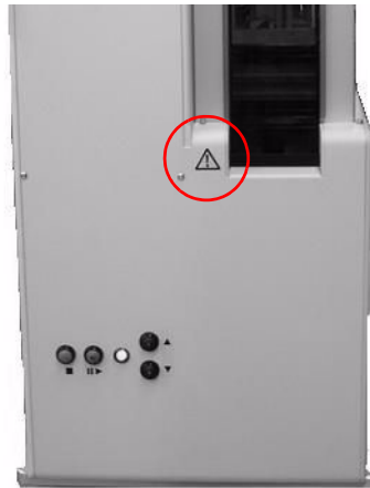
Fig. 19: Warning symbol at the belt stacker
