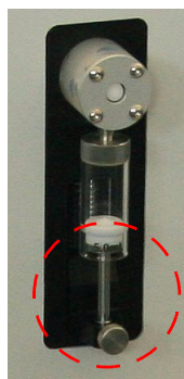
Fig. 111: Pump rod area, danger zone
