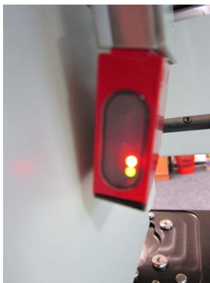
Fig. 2: Barcode reader's status LED continuously illuminated green, its decode LED continuously illuminated orange
