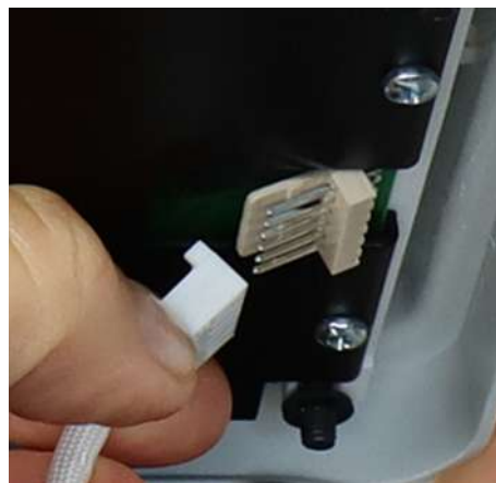
Fig. 9 Disconnecting the plug connection
