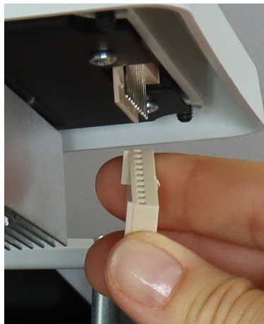
Fig. 9 Disconnecting the plug connection
