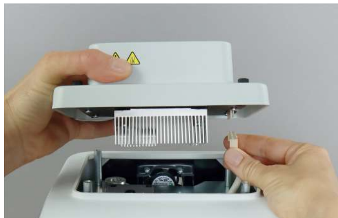
Fig. 8 Establishing the electrical connection between the basic device and the block module
