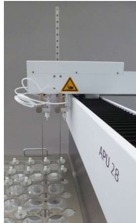
Fig. 8 Double channel system APU 28/1 S with 2 dosing heads and needles
