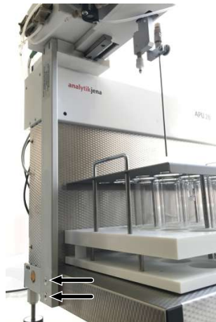
Fig. 15 Removing the transport lock
