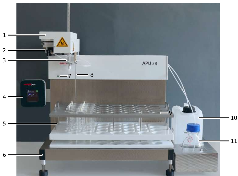
Fig. 7 Single-channel system APU 28 connect SPE comprising basic device APU 28/1 SPE and control module
