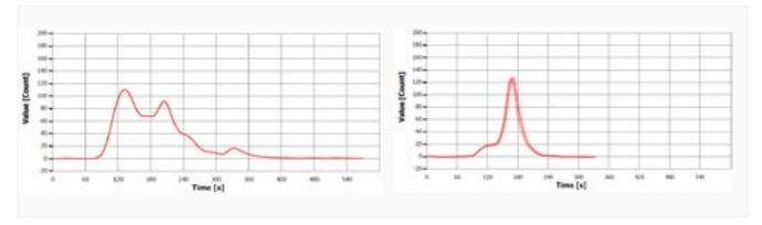
Figure 2: Typical TN measurement curve of adipic acid
