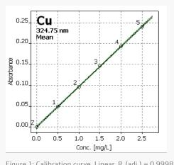
Figure 1: Calibration curve, Linear, R<sub>2</sub>(adj.) = 0.9998
