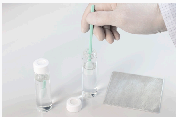
Figure 1a–b: Swab sampling on a test specimen, cross-wise in lanes
