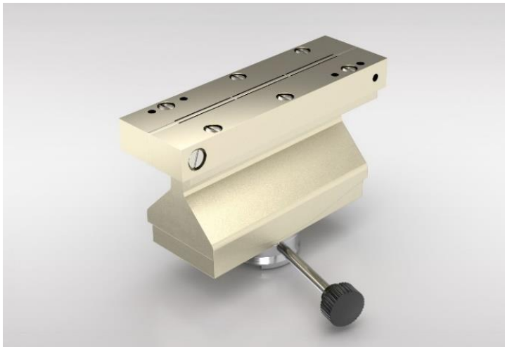
Figure 1: Design of the LPG burner head with two 100 mm long double slots, which are divided into three parts
