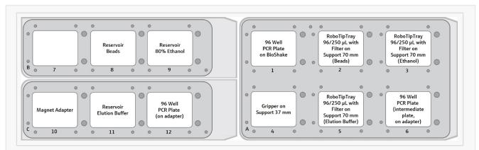
Figure 2: Graphical deck layout for Protocol – Double-sided Size Selection. The CyBio FeliX provides 12 deck positions on 3 movable decks. The upper decks B and C equipped with the required accessories are shown on the left, the lower deck A is shown on the right. The 12-column reservoir on position 8 is equipped with 2 mL AMPure XP beads per column.
